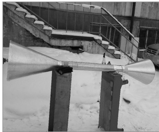
Fig. 3. Experimental setup for an icing wind tunnel.
