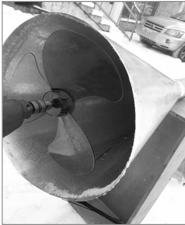
Fig. 3. Experimental setup for an icing wind tunnel.
